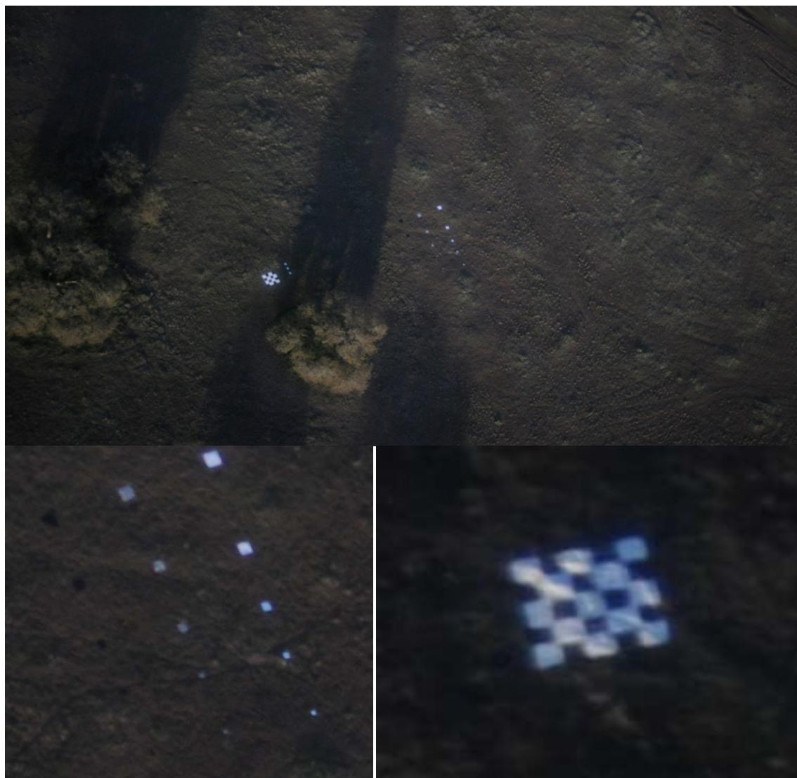
Figure 6. Photograph taken from an UAS during resolution tests at Camp Roberts, California, during December 2009. The upper photographs were taken with a 12 megapixel camera with resolution on the ground of 2.9 cm. The colored patches in the lower left photograph vary in size from 15 cm squares to 50 cm squares and are a magnified view of the upper photograph. The lower right photograph is a magnified view of a 2 m square checkerboard with each checkerboard square 40 cm by 40 cm.
