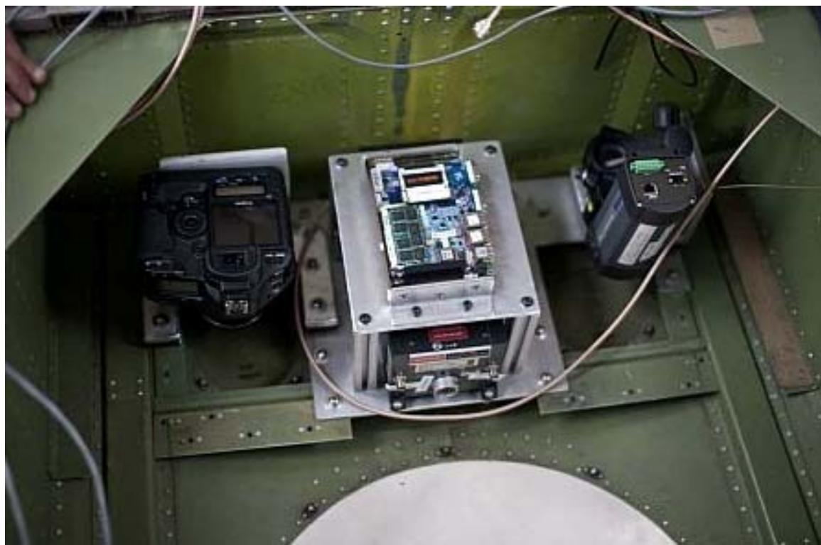
Figure 7. Camera mount and associated data storage and control devices that can be mounted as a module in a Twin Otter.
