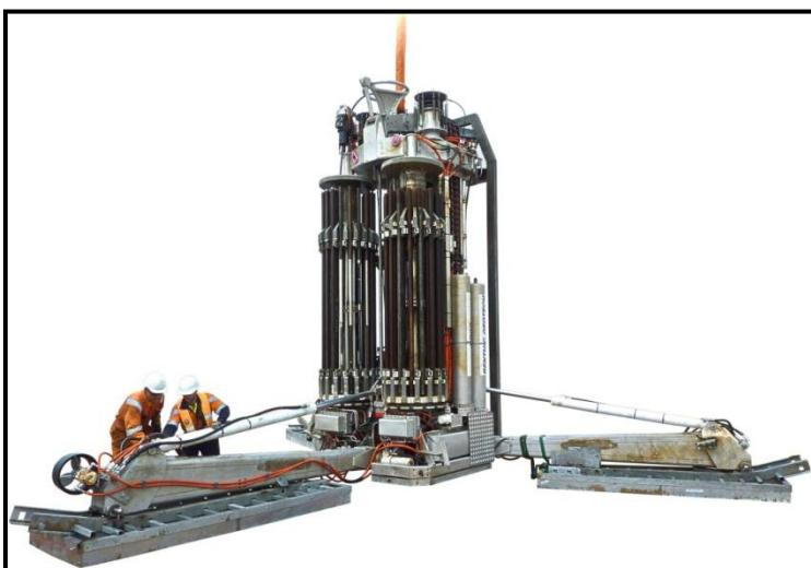
Figure 2.3-1 Schematic of Geotechnical Survey Acquisition with a Seabed Drilling System
